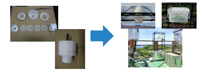
PBM by Tekran 1135 indicates the particle smaller than 2.5µm. To obtain the information of mercury in large particle (>2.5µm), sampling and analysis of particle matter using by quarts fiber filter is begun in continuous mercury monitoring site (Cape Hedo and Oga)
