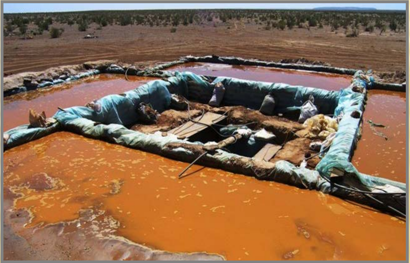
A group of four raised plastic-lined vats for cyanide leaching of gold-bearing tailings that are also mercury-bearing. In the middle is the sump into which gold leachate is routed by gravity via a set of plastic pipes. Dornogobi Aimag.(2006,
