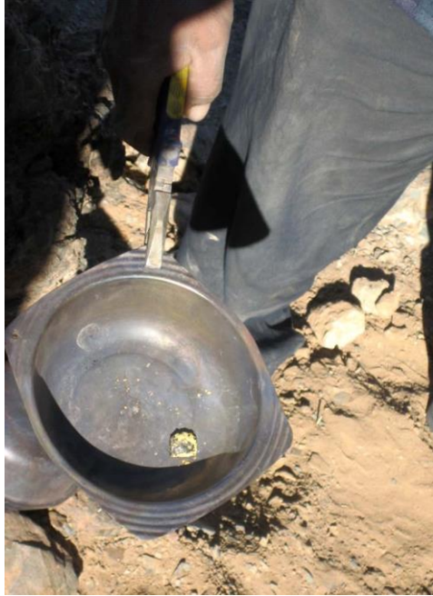
Mercury being driven off as invisible toxic Hg vapour by heating the Au Hg amalgam.
