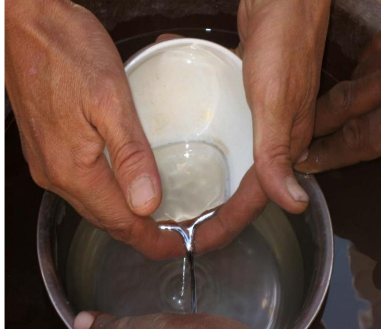
Metallic mercury in direct contact with unprotected bare skin of hands.
