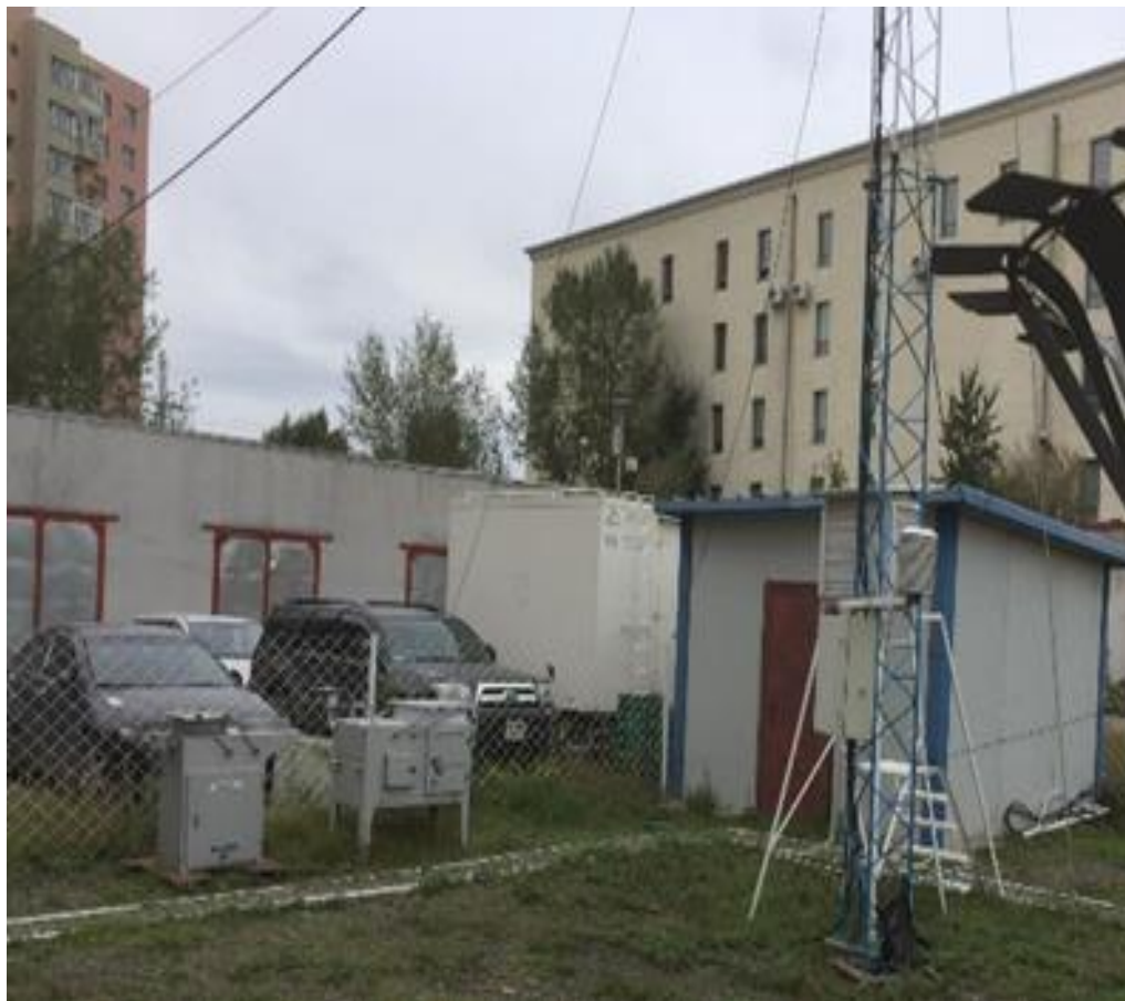
Mercury Deposition Sampler /CLEM/
